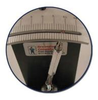
Wobble gaging provides a means for determining the compatibility of cross recesses in the heads of machine, tapping and wood screws with companion screw drivers and will indicate the point where deviation in the recess contours affect satisfactory driver engagement. Recesses which exhibit excessive wobble characteristics will cause poor screw drivability because of driver camout prior to attaining normal torque level, damage to recesses, and/or accelerated driver wear
